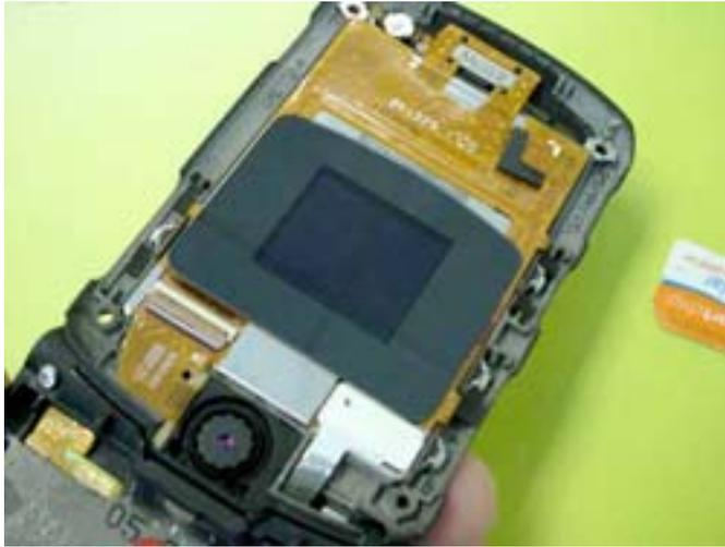
Pop off the connector here. This connect the keypad to the mainboard.
