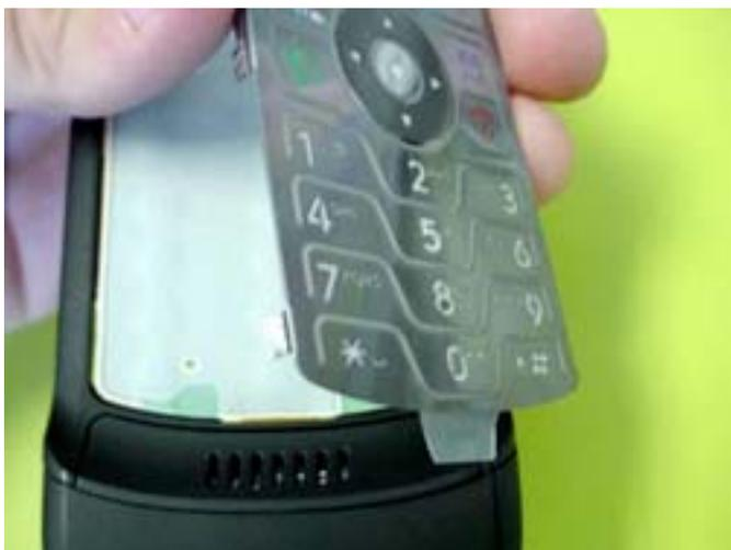
Now you see the keypad. If you need to replace that, it is stuck on with an adhesive. I am not going to take it off in this guide, since it won't go back on well, but all you do is get some tweezers or a knife under a corner, and pull it up like you'd pull gum off a shoe.
